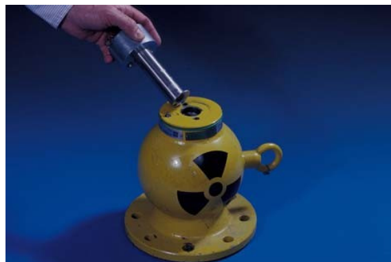
Lead radioactive source container with source holder removed (PHE)
